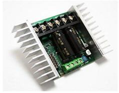
Sabertooth may be a dual channel motor driver capable of supplying 25 Amps to 2 motors, with peak currents up to 64 amps per motor.it are often operated for radio control, analog, TTL Serial or USB inputs. It uses regenerative drive and braking for efficient operation.
