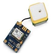
GPS module makes use of signals sent by satellite in space and ground stations on earth to accurately determine its position it's on earth. The GPS module for Arduino is a small electronic circuit that permits to attach to your Arduino board to urge position and altitude, also as speed, date and time on UTC (universal time coordinated).it uses the standard NMEA protocol to transmit the position data via interface.
