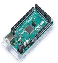
Arduino board is an Open Source microcontroller board which is based on At mega 2560 microcontroller. it is an open source electronics platform supported easy-to-use hardware and software. This Board is in a position to read inputs-light on a sensor, a finger on button or a twitter www.ierjournal.org
