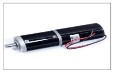
A gearmotor is an all-in-one combination of an electric motor and a gearbox. This makes it an easy, cost-effective solution for high-torque, low-speed applications because it combines a motor with a gear reducer system.
